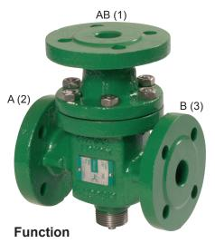
Without an actuator being installed, connection A-AB is fully open and connection B-AB completely closed, by means of a spring.
