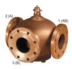
proportionally to the travel of the spindle, and when the spindle is pressed to the bottom, connection 3-1 is fully open and connection 2-1 completely closed.
